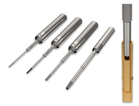
In some cases, probes can break inside of a receptacle. It can be challenging to remove damaged barrels especially in case of threaded probes without the correct tool. We can eliminate this problem with our BPET series. BITs have special left-handed threaded tips to make extraction simple. Just insert the tool and press down a little while turning it counter-clockwise, then remove the damaged barrel with ease.
